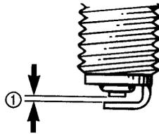
To maintain a proper functioning spark plug, keep the plug free of carbon. Remove carbon from the plug with a wire or pin, and adjust the gap to 0.24 - 0.28 inch (0.6~0.7mm) for good ignition. Use a thickness gauge to check the gap.
