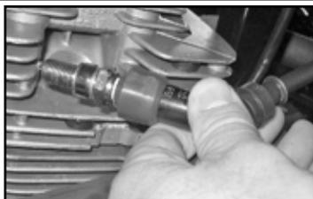
1. Remove the spark plug and reattach it to the spark plug lead.
