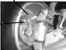
1. Try to move the vehicle backward and forward when the front brake is applied. If the front wheels can turn, adjust the front brake to lock the wheels securely.
