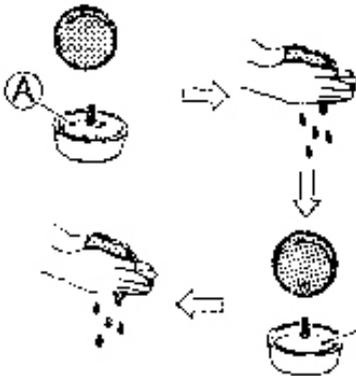
1. Fill a washing pan large enough to hold the element with a nonflammable cleaning solvent. Immerse the element in the solvent and wash it.
