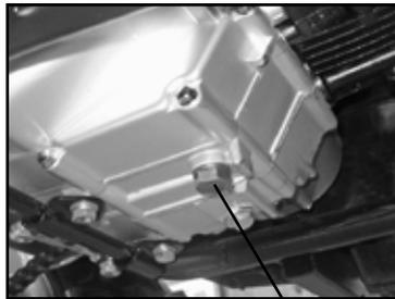
3. Remove the drain bolt and drain oil into proper container. Oil drain bolt
