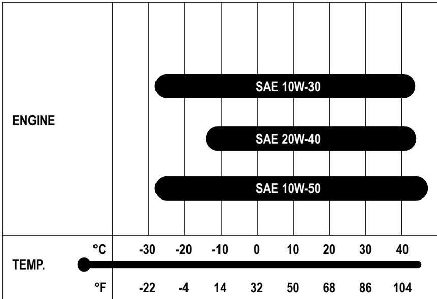
Use the chart to select a viscosity rating based on the temperature range in your area.
