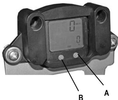
After power is turned on, press A to change between time, trip mileage or cumulative mileage.
