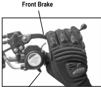
To stop the ATV, first release the throttle lever, then apply the rear and front brakes smoothly.
