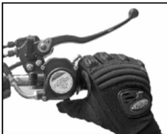
Release the rear brake lever and open the throttle gradually to move forward.
