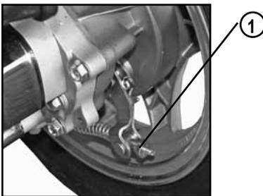
1. To make rear brake adjustment, turn rear adjusting nut (1) clockwise to increase and counter clockwise to reduce tension on the brake cable.
