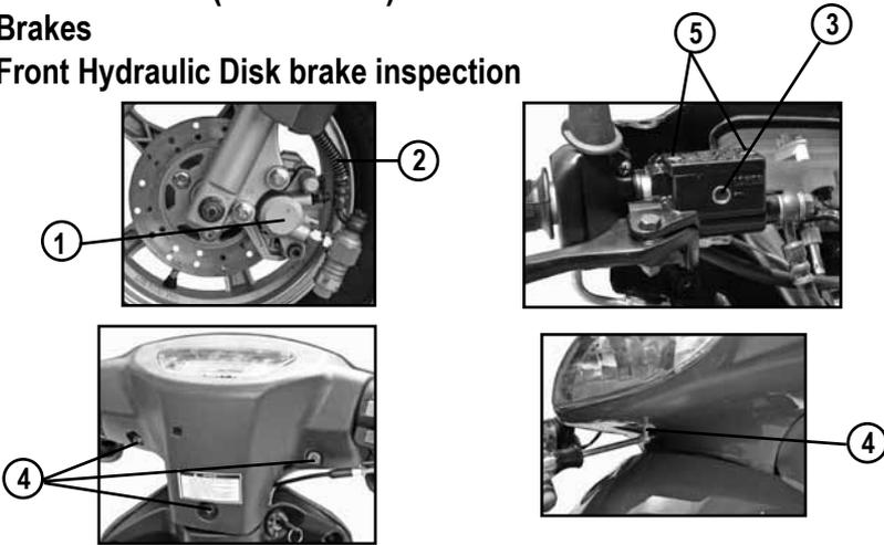
1. Inspect front disk brake caliper (1) for leakage. If brake fluid leaks, the safety of riding could be affected.
