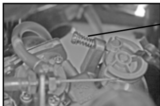
Engine Idle adjustment Screw
