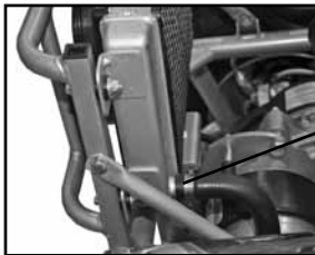
Remove hose to drain radiator fluid
