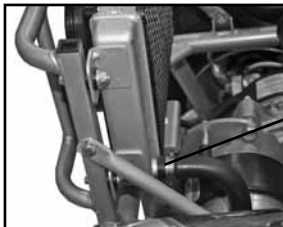
Remove hose to drain radiator fluid
